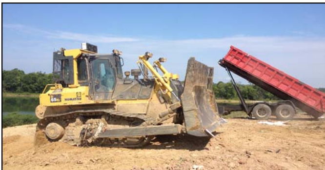
At the landfill, an Off Road Bulldozer begins to push dirt while a truck dumps a roll-off container.
